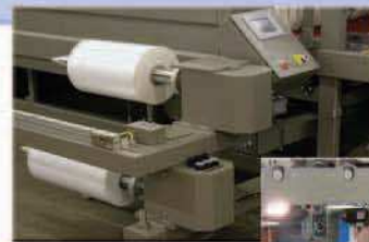
Roll-out film cutter assembly for easy maintenance.
