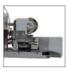
Trim saw ensures positive, precise sizing of bag top before it enters folder section.
