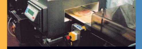
The Goring Kerr DSP 3 metal detector systems offer a high performance, cost-effective solution for process and package inspection. Every model provides the ideal QA means to implement your HACCP plans and incorporates the hygienic standards required in the food industry. Backed with more than 50 years experience, Thermo's Goring Kerr metal detector systems will assure your product to be metal contaminant free and protect your brand.
