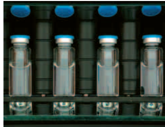
Two mirrors for bottom and cap inspection
