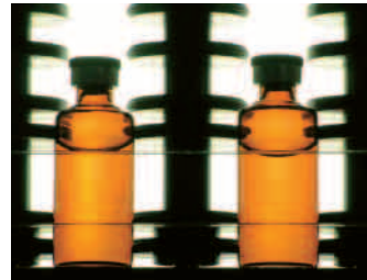
Background light in combination with Tyndall illumination
