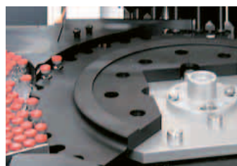
Tray unloader with segmented infeed starwheels
