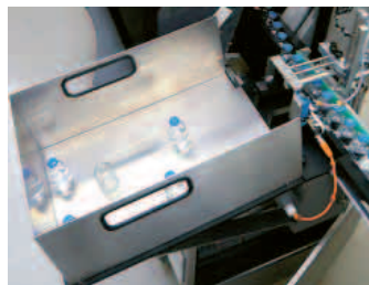
Separation of defects for bottles
