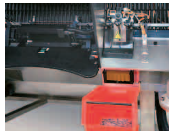
Separation of defects for small containers like syringes or cartridges
