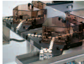
Y-Mag modules to separate two reject categories
