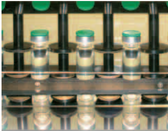
Particle inspection of liquid products against polarized background light, as well as cap, crimp and bottom control
