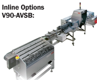
Bulk syringe feeding and orientation system in line with V90-AVSB
