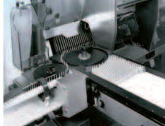
Infeed combination syringe/vial
