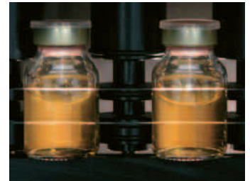
Special light to check albumin for microbial contamination
