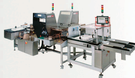
Inspection lines for lyophilized product in vials. Infeed: Bi-flow tables. Outfeed: High-speed tray loader MGZ-2
