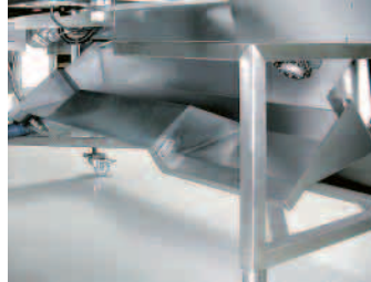
Bottom dust pan to collect dust, product debris and liquids in an easily accessible area
