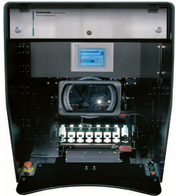
Ergonomic cockpit design reducing stray light and glare, touch screen HMI for all operating functions
