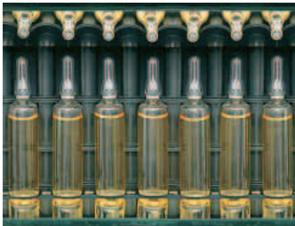
Tyndall light systems and inspection against dark background
