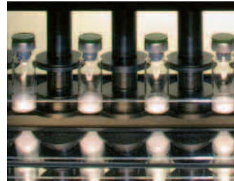
Disk rollers for presentation of lyo-filled vials at 75° inclination
