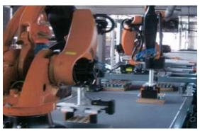
Robotic Case Turning and Positioning
