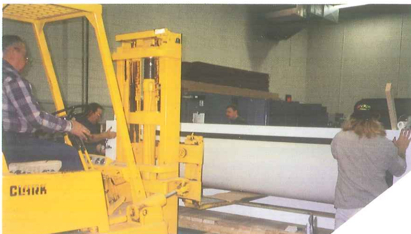
Large ceramic covered-roll being installed in station frame.
