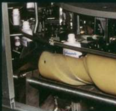
Line Shaft Drive into a Feed Screw
