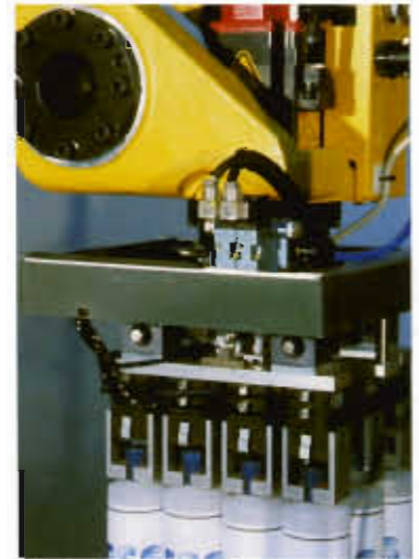
Custom End-Of-Arm Tooling with quick change features.
