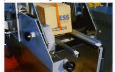
Ergonomically designed, large capacity, case magazine.
