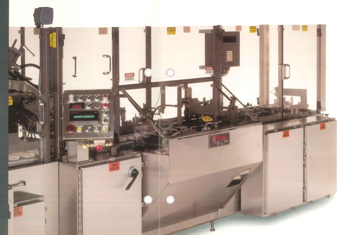
infeed capabilities. Many different infeeds are available, making the PSC especially well-suited to handle blisters (samples or hospital unit doses), bottles, tubes, transderm pouches, syringes, and many
