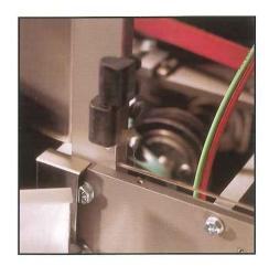
**SOLID, STABLE FRAME.** Made of 1" x 3" cold rolled steel. Welded and bolted design adapts to changing needs that's impossible with a cast frame. All holes are drilled and tapped, so bolts don't work loose.
