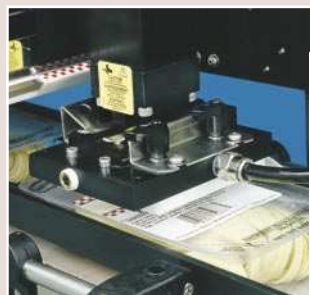
7 Non-contact or gentle-contact application accurate to \pm 0.03 ".
