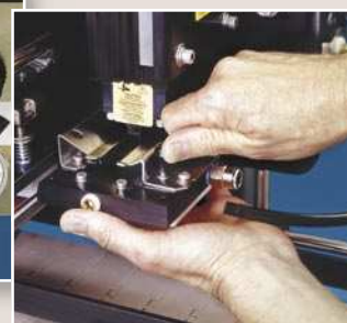
6 Quick-change tamp pad allows for easy replacement to accommodate different label sizes.
