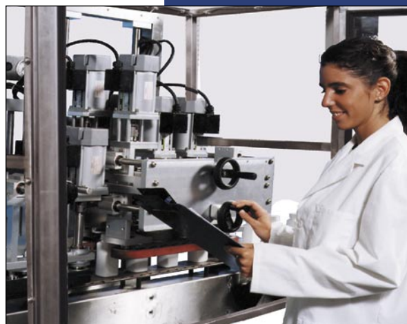
Quick handwheel height and width adjustment with position indicator
