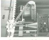
For cartridge or cylinder-type desiccants. Speeds to 100 BPM. Single or multiple desiccants per container. Starwheel design. Changeovers completed in minutes.
