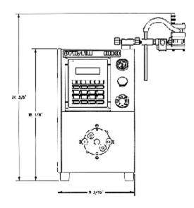
Air Requirements: 80 PSI @ 1 SCFM Electrical Requirements: 110 VAC 50-60 Hz. @ 15 AMPS Shipping Weight: 80lbs.
