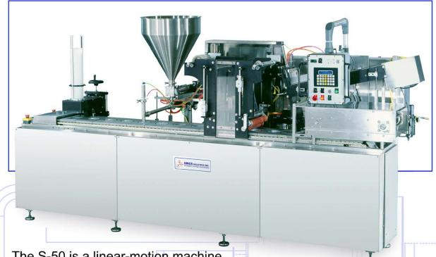
The S-50 is a linear-motion machine. Fills, seals roll film or die-cuy lid and over-caps. Speeds from 30 to 240 containers per minute.
