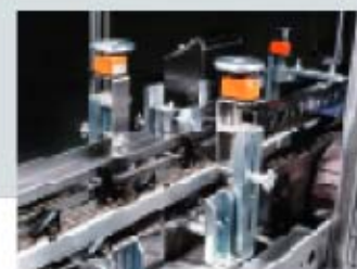
Optional digital readouts on adjustments are used for consistent and faster carton size changeovers.
