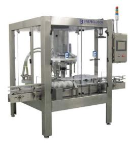
The new **Biner Ellison RVF Series** machines set new standards in design, speed, safety, productivity, efficiency, and price. The RVF Series is an impressive line that provides precise volumetric filling of viscous and semi-viscous products utilizing our proven "Synchronized Pump & Turret" metering system. The new design incorporates an overhead drive system and powered nozzle height adjustment with job memory.
