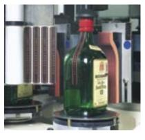
Application of an additional self-adhesive label with cold-glue labeller
