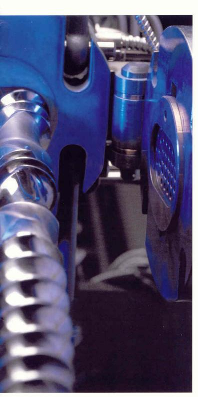
The FTX Twin-Screw Extruder effectively converts a wide range of raw plastics into custom-made compounds ready for final product applications.
