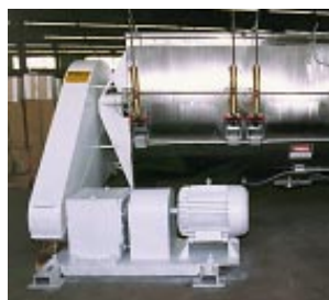
Side-by-side chain drive
