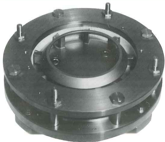
View looking into the microcut head and impeller. For use with Models 4200 and 1700.
