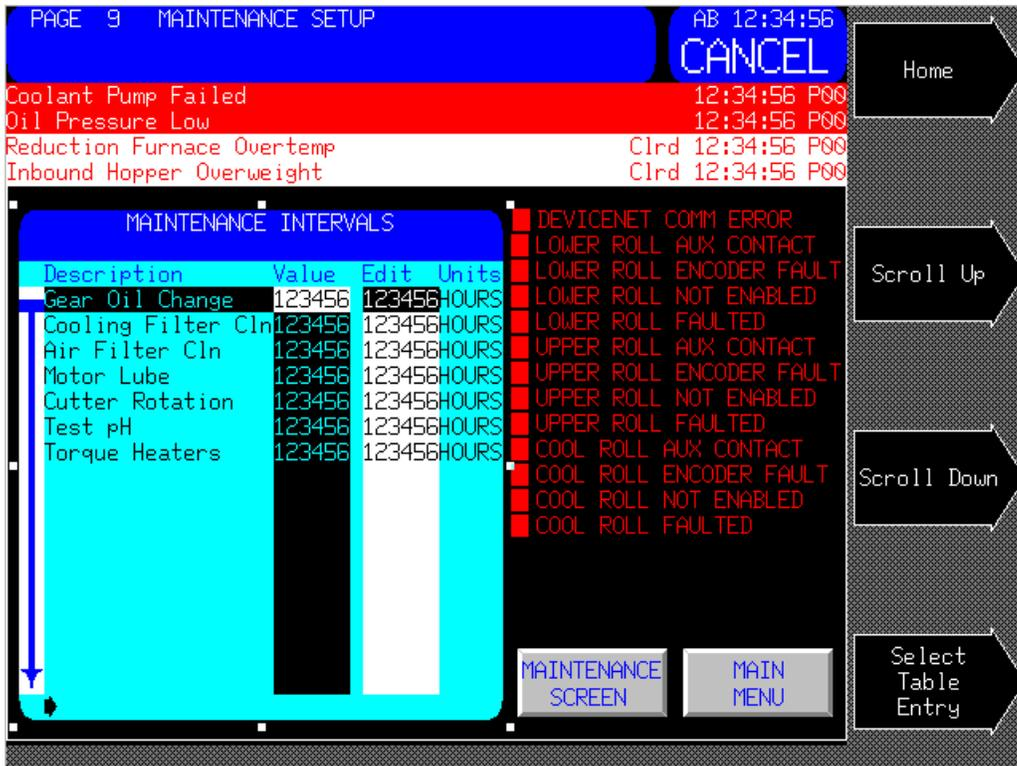
Another type of button that you will see is a parameter button. These buttons allow the operator to adjust various operating parameters. To edit a parameter, select the parameter button, and then select the proper parameter by using the Scroll Up and Scroll Down specific commands.
