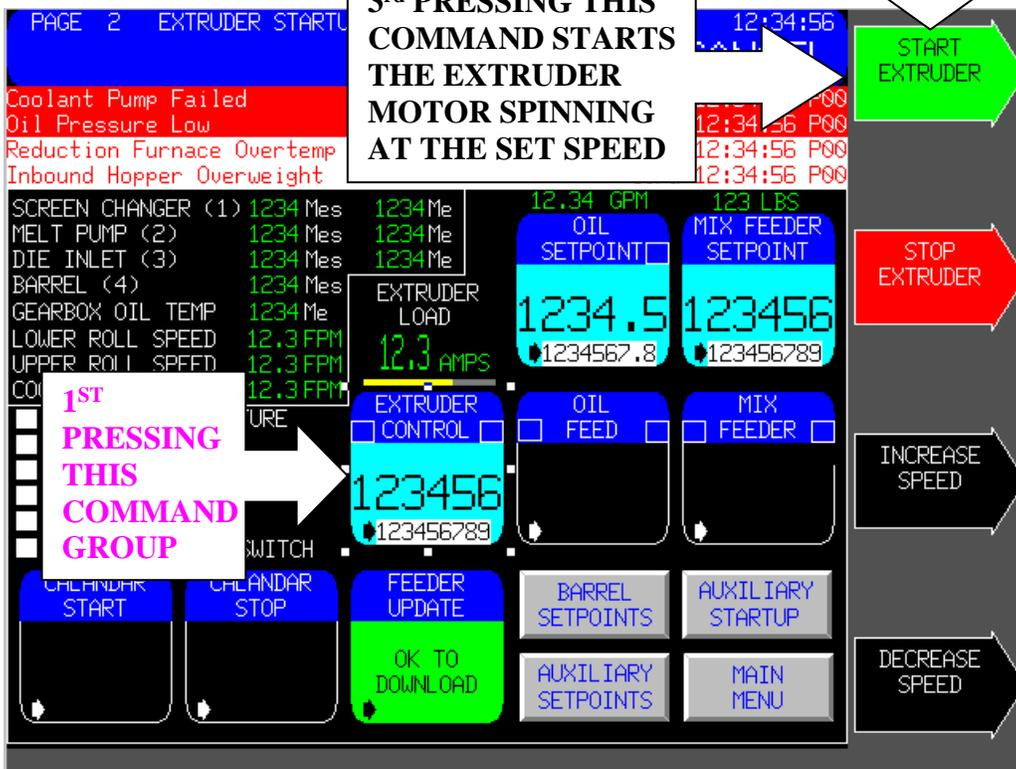
other options like Increase Speed and Decrease Speed. When any of the specific commands are activated the named function immediately activates as long as all of the safeties are ok.
