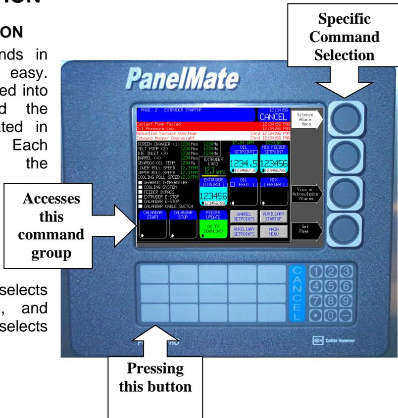
Also, this operator interface is not a touch screen because of the nature of plastics work. The screen would quickly get too dirty to operate.
