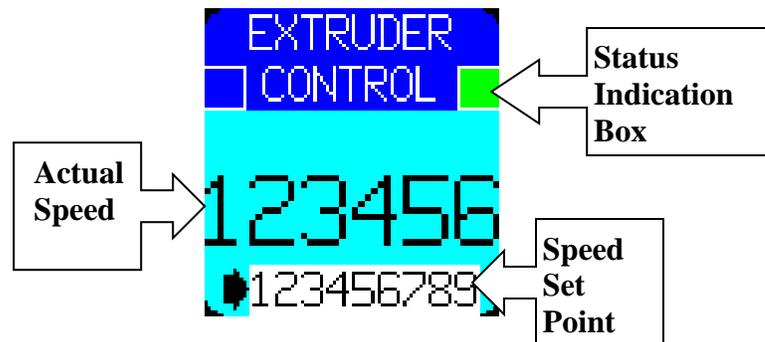
2. **Analog Command Groups** – Analog Command Groups are a way to set the limits and operating parameters for various processes on the machine. Pressing one of these buttons brings up the Change Value specific command, and allows the operator to change the named value. An example of an Analog Command Group is Barrel Temperature Setpoint.
