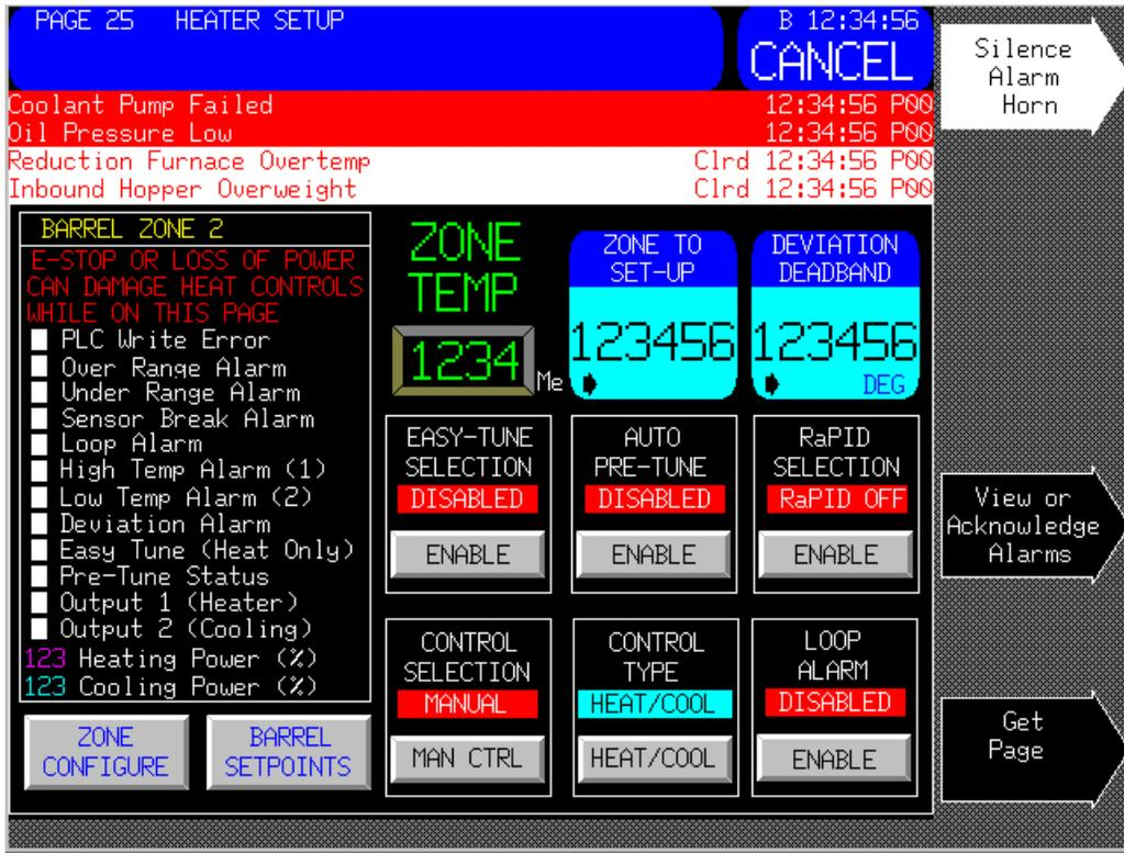
1. **Heater Setup** – The heater setup screen is used to modify each individual zone’s various operating characteristics. Once a zone is selected to be setup all of the information on the screen applies to the zone selected.
