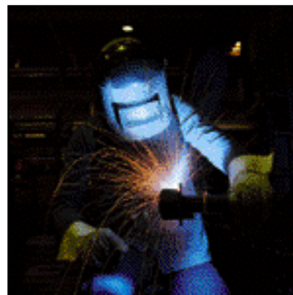
GTAW and GMAW welding processes are utilized on nozzles and end frame reinforcing bars, respectively.
