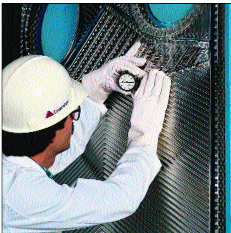
Draw depths of plate chevrons are meticulously monitored.
