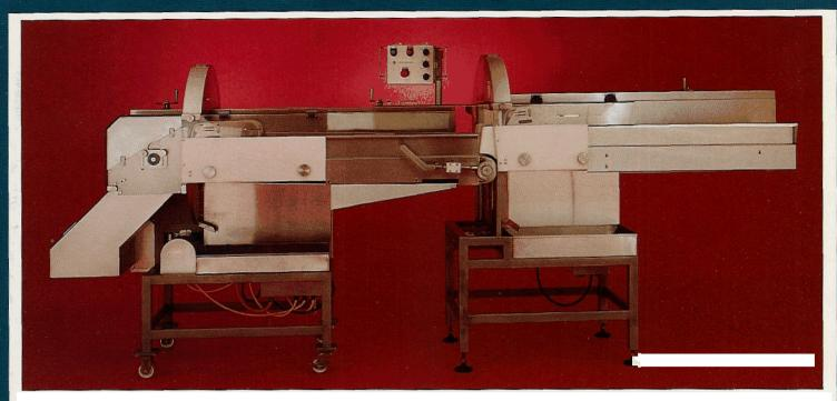
The Auto-Slicer provides high speed processing with consistent portion sizes for a wide variety of raw or precooked products including:
