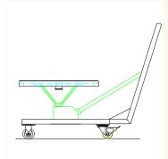
The ROMAN Filter has a unique cart assembly used for both lowering the filter plate and moving the filter from location to location. In addition, only one cart assembly is needed for all ROMAN Filter sizes, minimizing required storage.
