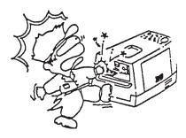
■ **NEVER** touch output terminals during operation. This is extremely dangerous. Always stop the machine when contact with the output terminals.
