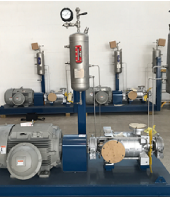
RS-C Multi-Stage with API Plan 52/Tandem Seals
