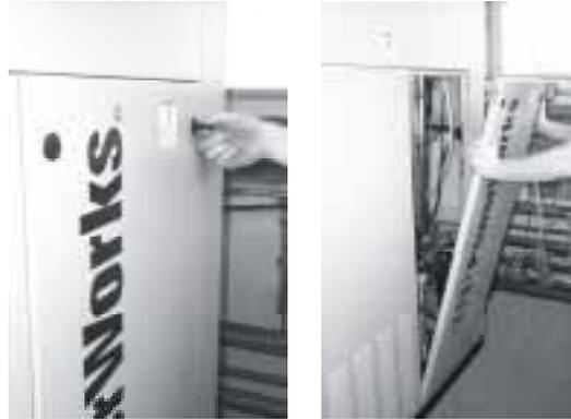
*Figure 40. Removing the right rear enclosure panel*
