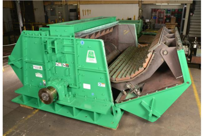
*Hydraulic doors make accessing critical wear parts easy.*
