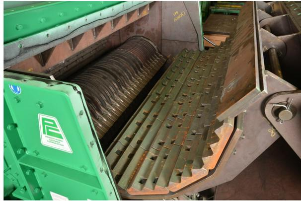
Top left: Shallow breaker block design reduces coal build up and increases crushing surface.
