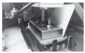
Mandril plunges blank through tooling cavity and the result is a completed corner glue, cornerlock, or simplex tray.
