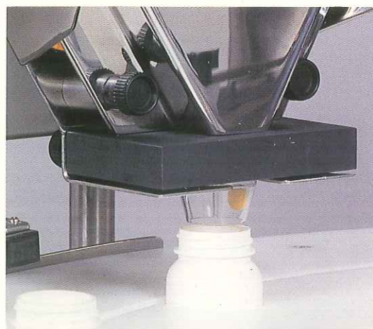
Power lift at the touch of a button adjusts the Monocount for different bottle heights
