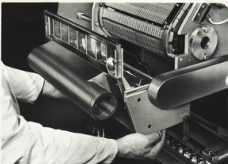
Head mechanism slides out of machine for ease of cleaning
