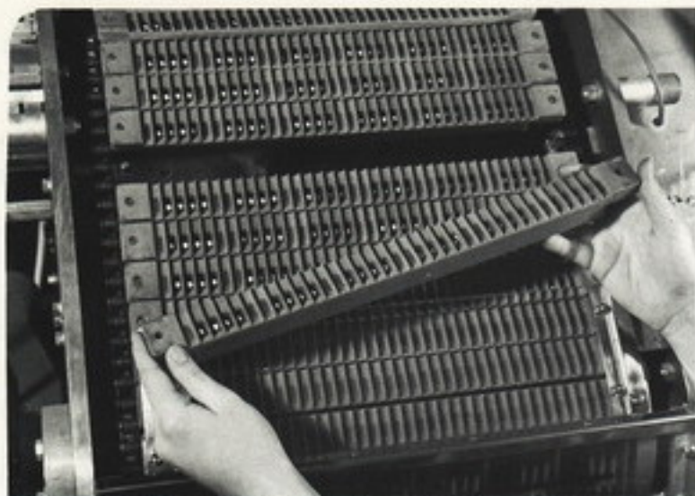
Slat are easily removable - no tools required
