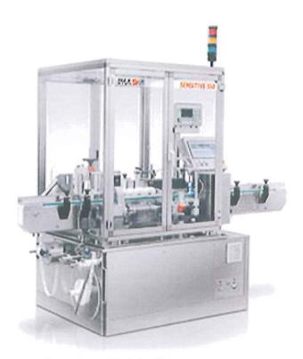
Sensitive 350 is a completely automatic labelling machine, designed to apply self-adhesive labels on the body of cylindrical containers in glass, metal or plastic with a maximum speed of 350 pcs/min.
