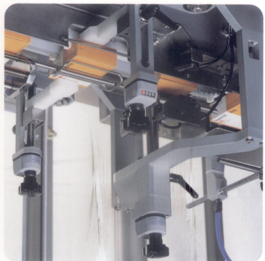
A DOUBLE ECCENTRIC CONTINUOUS MOTION DEVICE THAT FOLDS THE LABELS AS THE CARTONS PASS.
