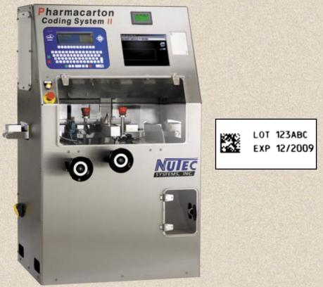
The Pharmacarton Coding System II is designed for in-line, high resolution digital printing of lot, expiration, and bar codes for pharmaceutical and medical cartons. This new design overcomes the problem of printing high density bar codes and 2D codes in line by totally controlling the carton during the print and vision process. The PCS offers true ANSI / ISO on-line bar code grading functions that provide a quality tool to qualify code print and readability.
