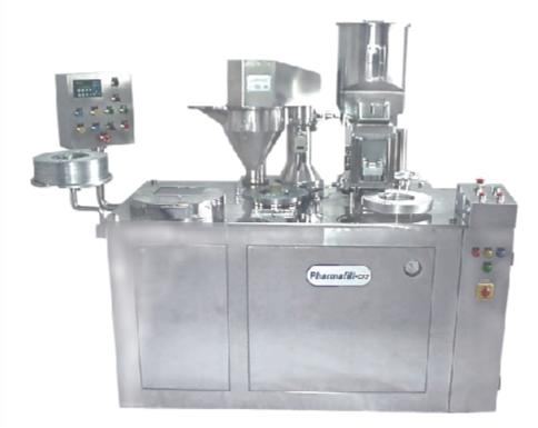
The **PHARMAFILL-CF2** machine is the latest in our range of high speed capsule filling machines. It is comparable to the best because of its outstanding features, both functional and mechanical. With an output of 30,000 capsules an hour, it is suitable for filling capsules of all sizes with powders, pellets or granules.
