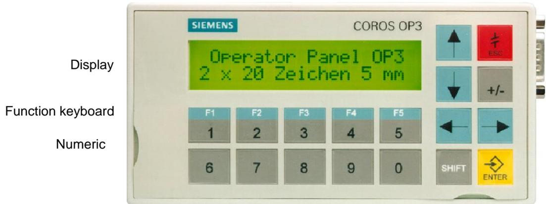
The OP 3 operator panel is for displaying and accessing faults that have occurred.
