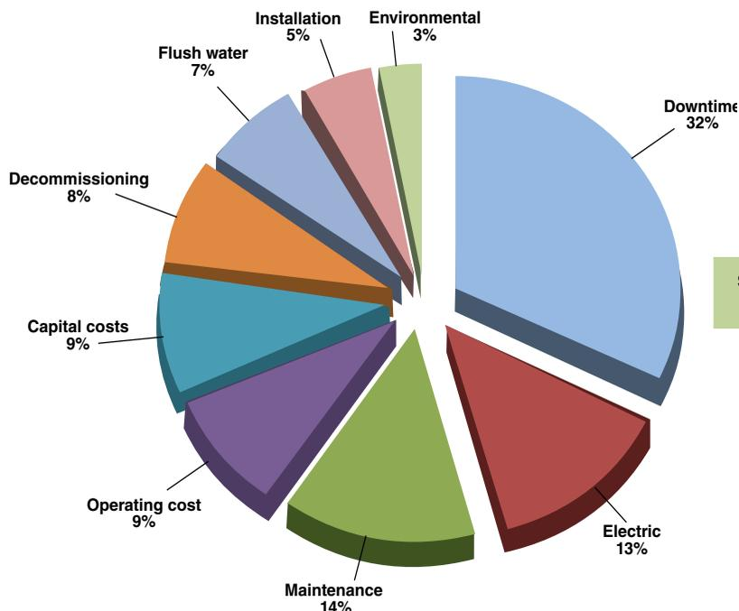
**FIGURE 2.** Initial capital costs represent a small fraction of the total lifecycle costs for process equipment. Operating costs, maintenance and cost of downtime can contribute more heavily to the total
