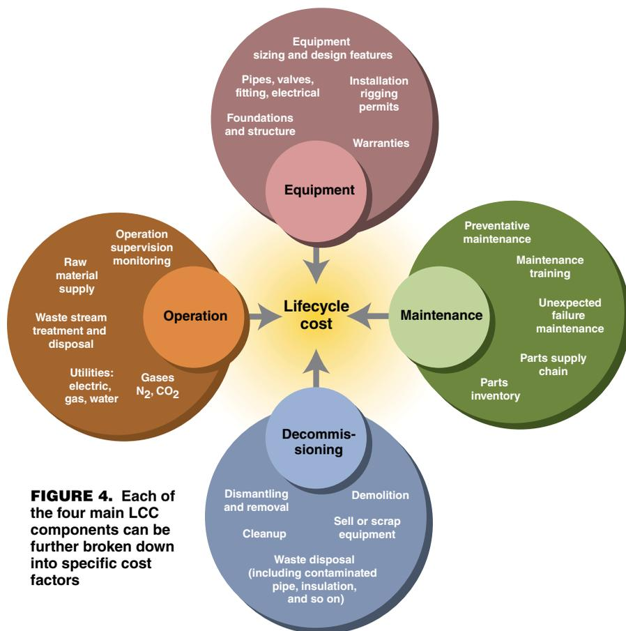
**FIGURE 4.** Each of the four main LCC components can be further broken down into specific cost factors
